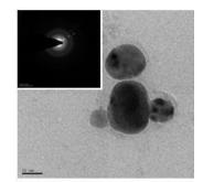
Fig. 4. HR-TEM image of Au nanoparticles
